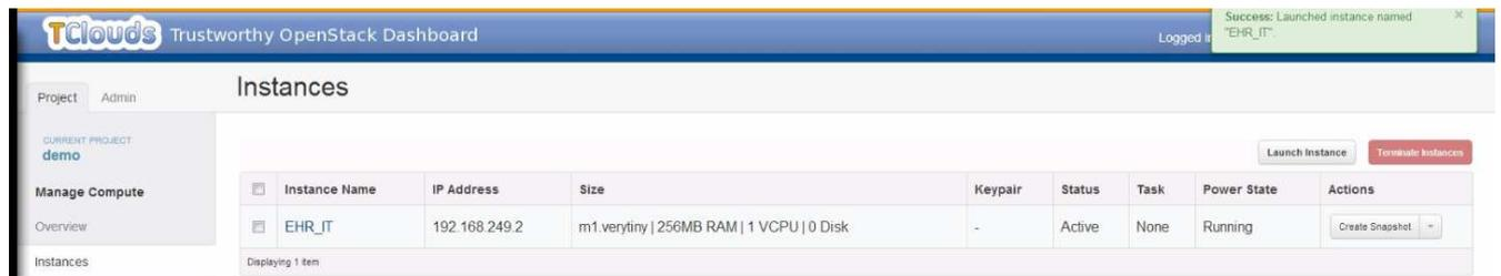
Figure 59 - Deployment of EHR\_IT VM. Please notice: I4 integrity level, TVD-healthcare and IT location
